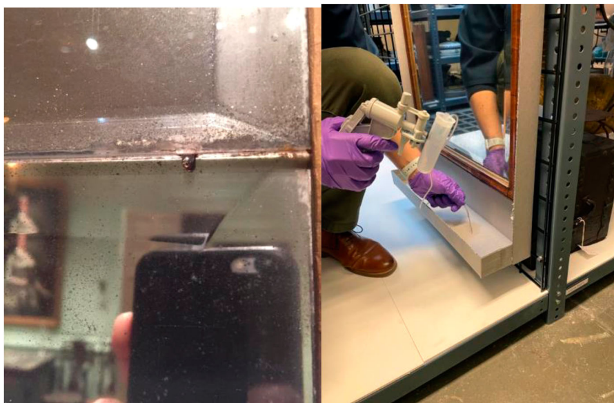
Figure 1. Mercury droplet as it forms on the seam of a looking glass (left). Preventive conservation staff clean up liquid mercury using a “Mercury Spill Control Station” kit (right). A manual vacuum gun lifts and encapsulates mercury droplets. The kit also contains a mercury sorbent, which helps to clean the vacuum reservoir by turning the mercury into a solid waste.
