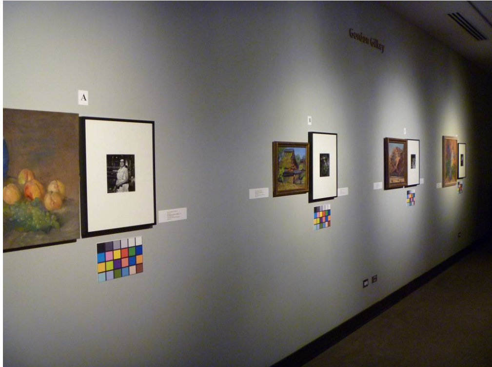
Figure 10. Gilkey Gallery with the four clusters of artwork arrayed along one wall. Each cluster was lighted with a different PAR38 lamp, lamp A (on left) through to lamp D (on far right). (Photo by PNNL.)
