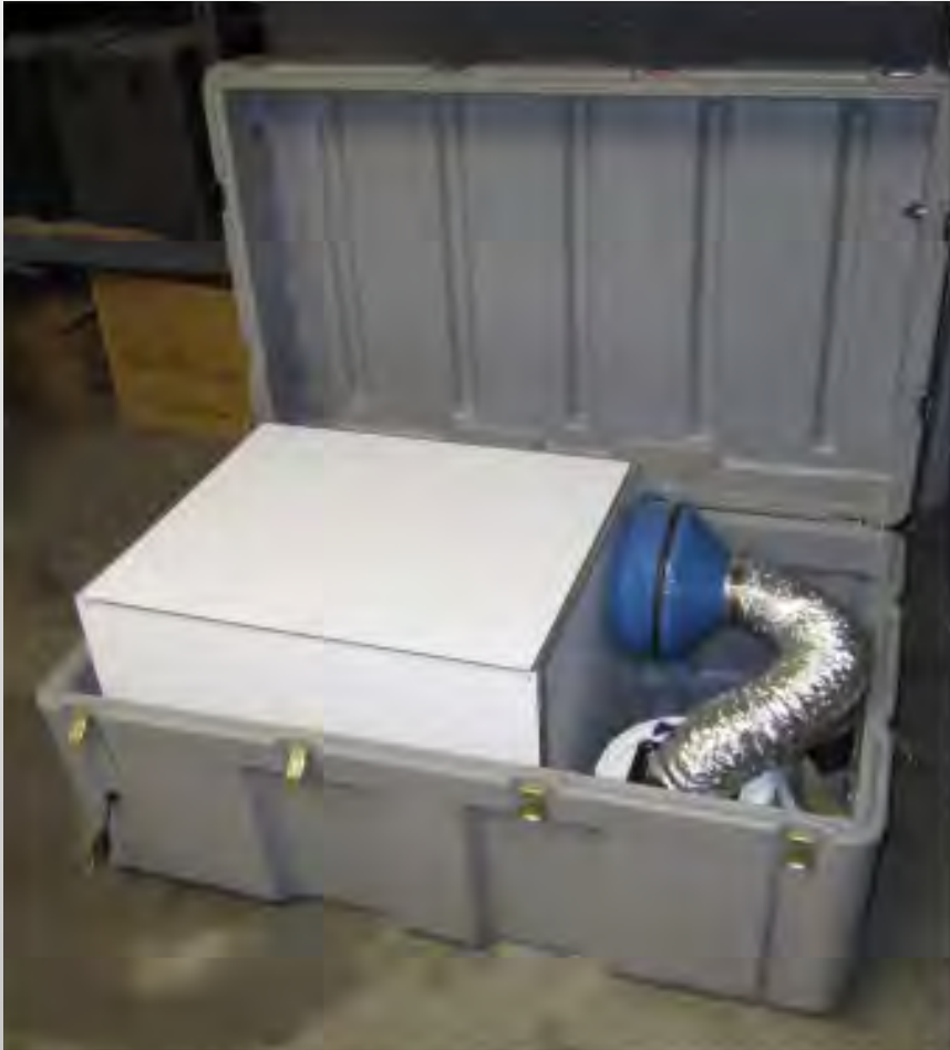
© Government of Canada, Canadian Conservation Institute. CCI 128941-0004 Figure 5. Example of a small conditioning chamber.
