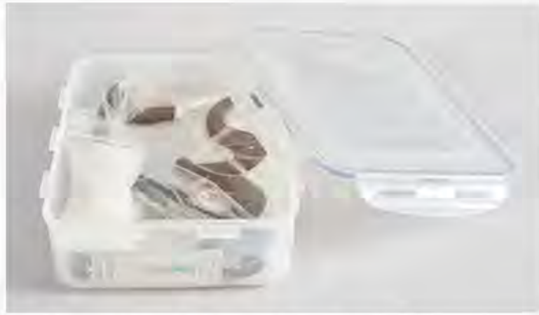
© Government of Canada, Canadian Conservation Institute. CCI 126258-0005 Figure 13. These iron objects are packed for dry storage in a food container with silica gel and an RH indicator card.
